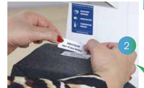
(2) Correct label positioned to cover the incorrect heat-sealing
